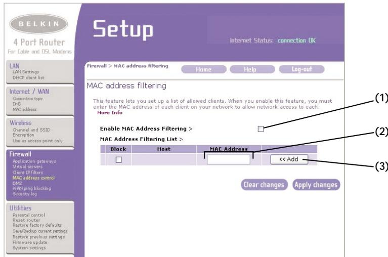
To enable this feature, select “Enable MAC Address Filtering” (1). Next, enter the MAC address of each computer on your network by clicking in the space provided (2) and entering the MAC address of the computer you want to add to the list. Click “Add” (3), then “Apply Changes” to save the settings. To delete a MAC address from the list, simply click “Delete” next to the MAC address you wish to delete. Click “Apply Changes” to save the settings.
