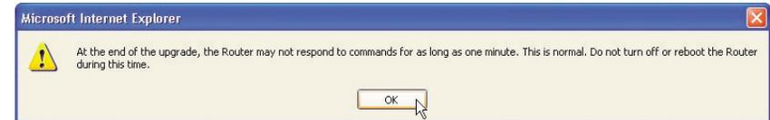
6. A 60-second countdown will appear on the screen. When the countdown reaches zero, the Router firmware update will be complete. The Router home page should appear automatically. If not, type in the Router's address (default = 192.168.2.1) into the navigation bar of your browser.
