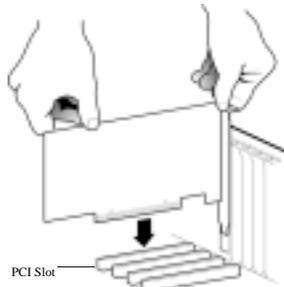
Be sure the bracket is lined up properly, then screw the bracket into the computer using the screw you removed with the cover plate. Be sure that the back end of the card (smaller gold finger area) is properly seated into the connector.
