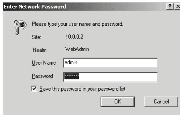
If you are not prompted for a **User Name** and **Password**, do the following in this order: Recheck all connections; restart the modem and computer; and reset the modem by inserting a paper clip into the **Reset** pinhole in the modem's back panel and pressing it three times.
