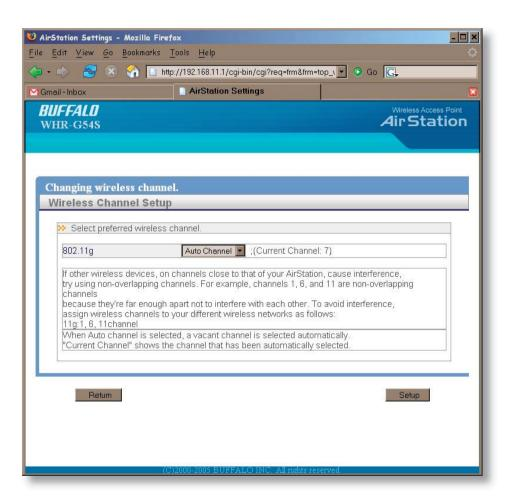
This page is available from *TOP* by selecting *Wireless channel*. With *Auto Channel* selected, your AirStation will choose the best channel available. *Current channel* will show the channel that your AirStation is currently using.
