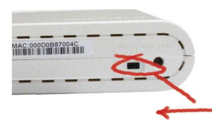
This AirStation supports quickly changing the product from a wireless router to a conventional access point.
