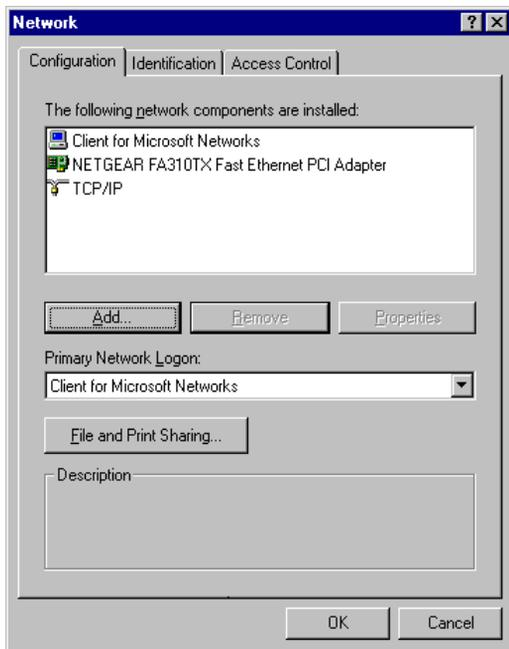
You must have an Ethernet adapter, the TCP/IP protocol, and Client for Microsoft Networks.
