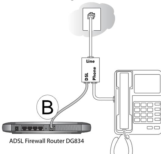
**Figure 3-5: Connecting the DG834 ADSL router to an ADSL microfilter and phone**
