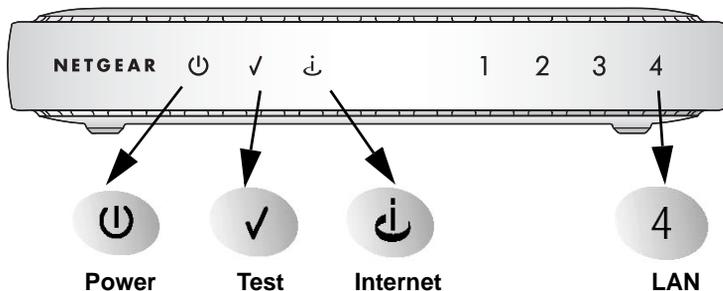
**Figure 2-1: DG834 Front Panel**
