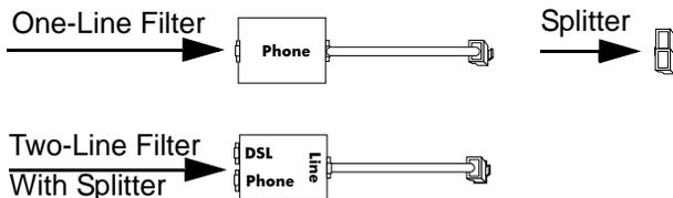
**Figure 3-3: ADSL microfilters**
