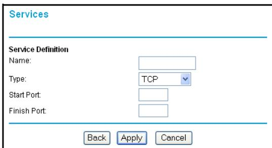
The screenshot shows the 'Add Services' menu. It has a 'Service Definition' section with the following fields: 'Name' (text input), 'Type' (dropdown menu with 'TCP' selected), 'Start Port' (text input), and 'Finish Port' (text input). At the bottom, there are three buttons: 'Back', 'Apply', and 'Cancel'.
