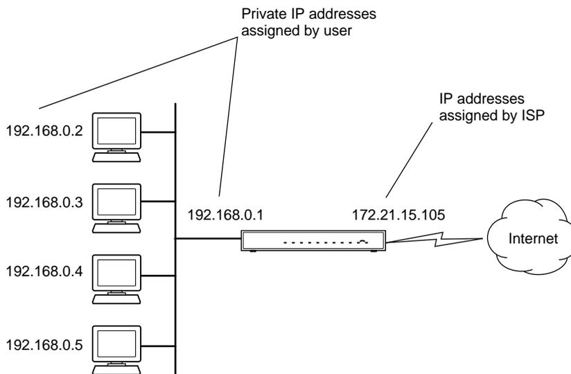
**Figure 7-3: Single IP Address Operation Using NAT**
