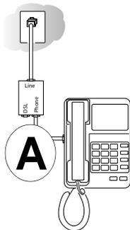
**Figure 3-4: Connecting an ADSL microfilter and phone**
