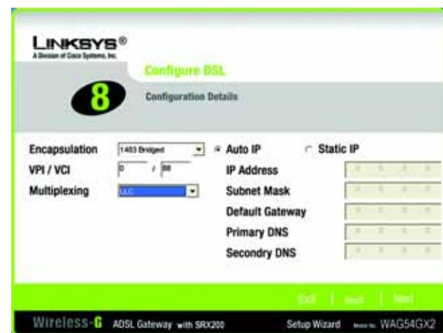
Figure 5-12 : Ecran Configure DSL - 1483 Bridged
