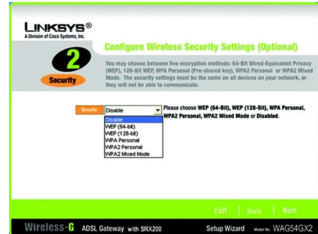
Figure 5-18: Setup Wizard's Configure Wireless Security Settings Screen
