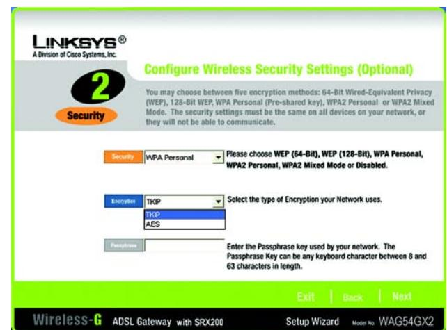
Figure 5-19: Setup Wizard's Wireless Security - WPA Personal Screen
