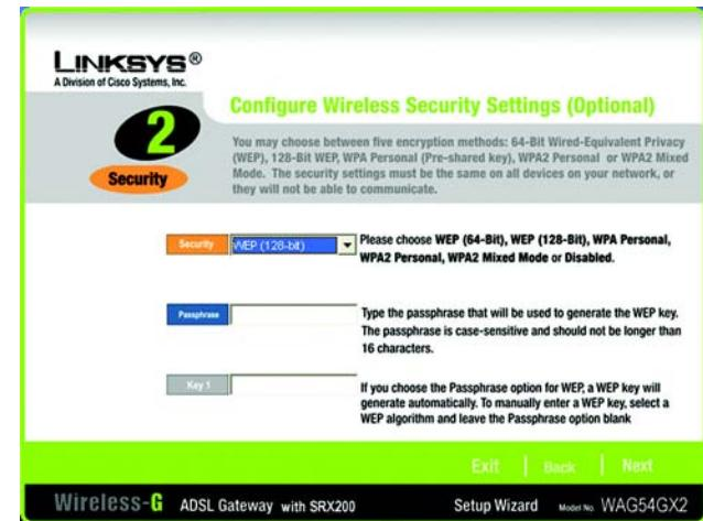
Figure 5-23: Setup Wizard's Wireless Security - WEP (128-Bit) Screen
