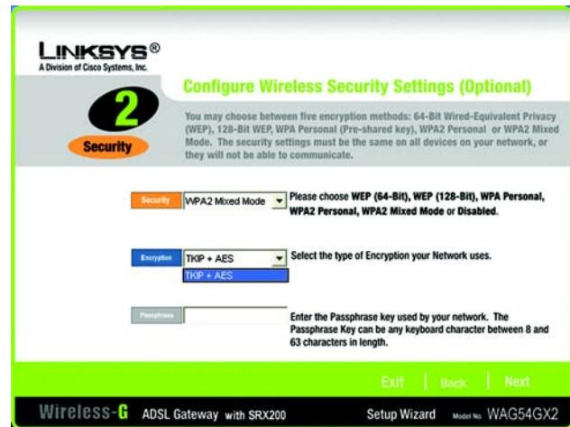
Figure 5-21: Setup Wizard's Wireless Security - WPA2 Mixed Mode Screen
