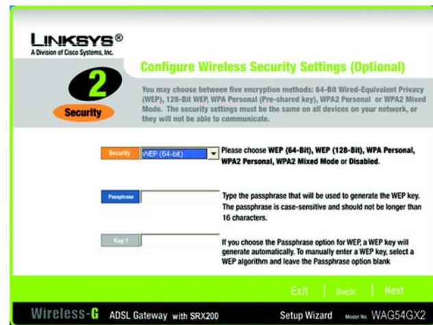
Figure 5-22: Setup Wizard's Wireless Security - WEP (64-Bit) Screen
