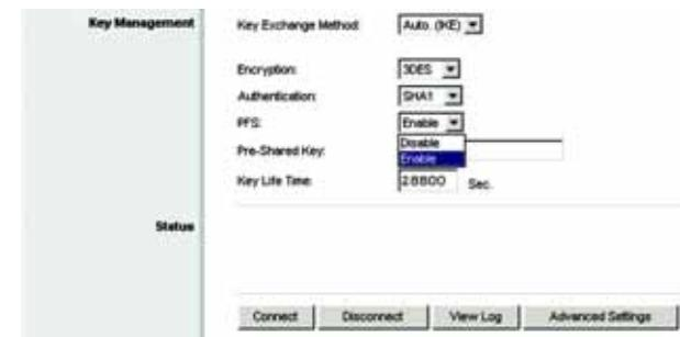
Figure 6-29 : Key Exchange Method - Auto (IKE)
