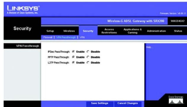
Figure 6-26: VPN Passthrough
