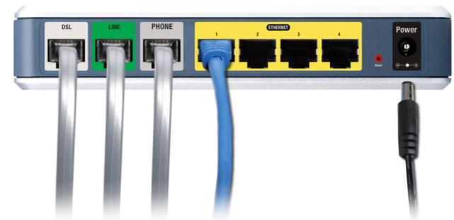
Figure 4-5: Connect the Power
