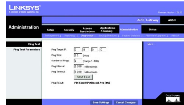
Figure 5-32 : Ping Test (Test Ping)
